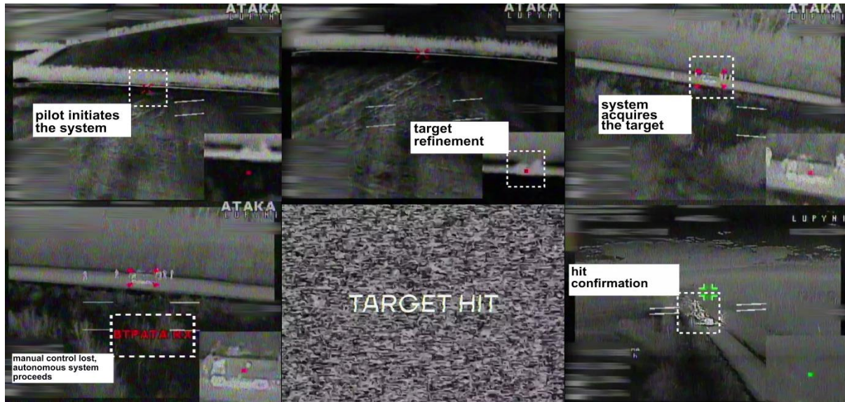
Image: TFL-1 equipped FPV Drone performing Terminal Guidance
